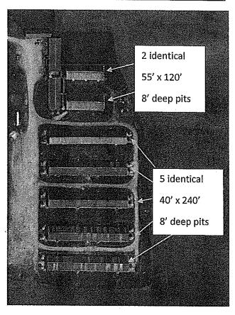
This swine facility utilizes concrete slats in the building, with all waste contained & stored in the 8' deep pits under the buildings. The waste is then land applied using a flexible drag hose reel to adjoining fields. An operator is at all times in view of the land application equipment in case of equipment failure.
